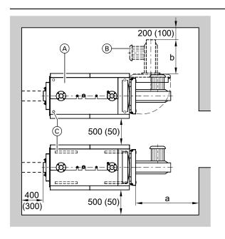
Observe the stated dimensions to ensure straightforward installation and maintenance. Where space is tight, only the minimum clearances (dimensions in brackets) need to be maintained. In the delivered condition, the boiler door is fitted so it opens to the left. The hinge pins can be repositioned so the door opens to the right.
