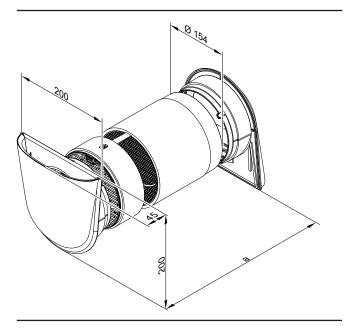
a Min./max. wall thickness depends on the combination of wall sleeve and external wall cover used.
