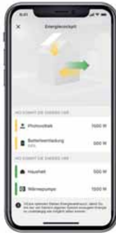
With the energy cockpit in the ViCare app, users can keep track of the energy flows in their home.
